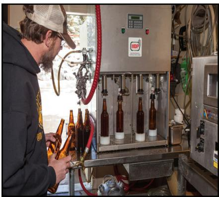
Assistant Brewer JJ Miles readies clean bottles to be filled and capped by the bottler and assures that the labeler mechanically adheres labels to clean bottles.
